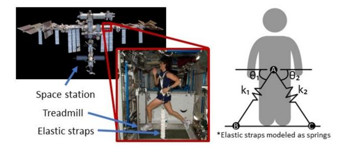
1) a) On the point below, draw a free body diagram for point A. Denote the force in spring AC as  $F_{AC}$ , the force in spring AB as  $F_{AB}$ , and the reaction force as  $F_P$ .
